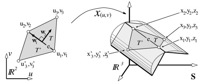
Figure 5: *Approximating the curvature around an edge  $e$ . The points of  $e$  can be considered to be cylindrical, with a null curvature  $\kappa_{min}$  associated with the direction  $\mathbf{w}_1$  of  $e$ , and a maximum curvature  $\kappa_{max}$  associated with a direction  $\mathbf{w}_2$ , orthogonal to  $\mathbf{w}_1$*
