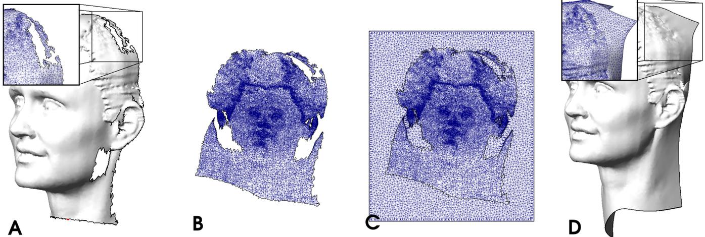
A: Due to shadows, scanned meshes often have complex holes and irregular borders. B: a global parameterization of the surface is computed. C: filling the holes and extrapolating the borders become 2D problems in parameter space. D: The locations of the new vertices in 3D space are computed by approximating a minimal energy surface (MES).
