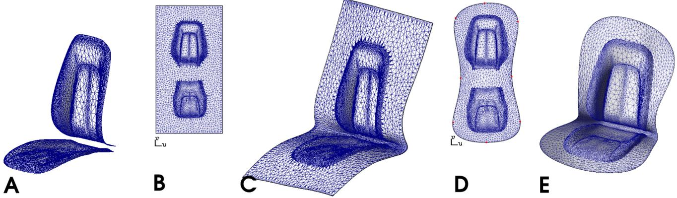
Figure 1: *Extrapolation and border editing in parameter space. A: original surface; B: constrained triangulation of the parameter space; C: extrapolating a minimal energy surface; D: the border has been edited and the constrained triangulation reconstructed; E: resulting surface: changing the border in parameter space means cropping a “virtual” surface, extrapolated from the initial surface.*
