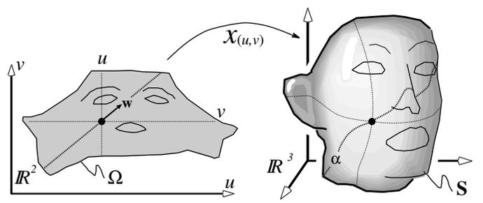
Figure 3: Computing directional curvatures on a surface.
