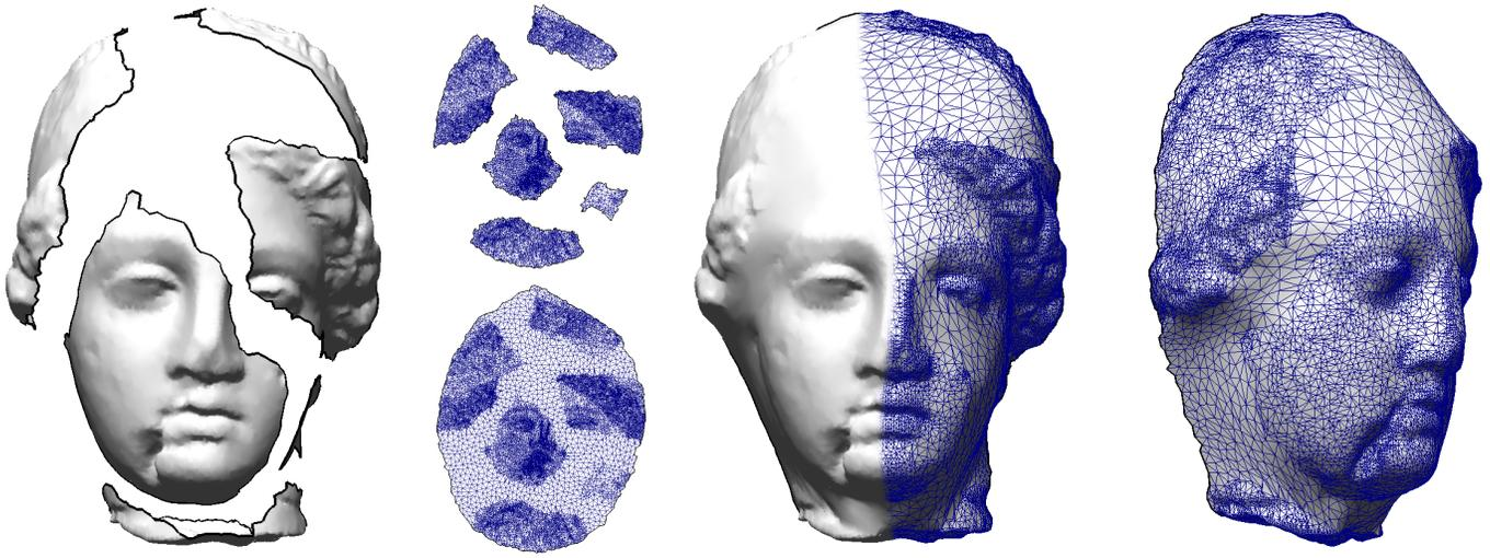
Figure 6: *Generating a complex blending surface. The charts are parameterized, the user arranges them in parameter space, a constrained Delaunay triangulation is computed, and the new vertices are optimized by minimizing the discrete MES criterion.*
